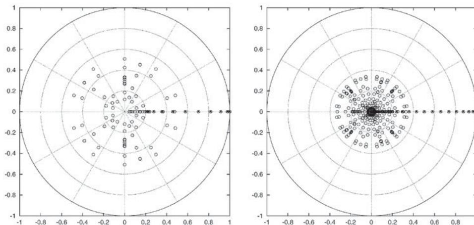
Figure 2. Spectrum of  $\hat{\mathcal{P}}_{\epsilon,S_2}$  for the linear shear  $S_2$  (○) and values  $\{d_{\epsilon,(j,0)}^{(N)}\}_{j=0}^N$  (▲). Parameters are  $N = 20$  (left),  $N = 40$  (right) and in both cases  $\epsilon = \log(N)/N$ .
