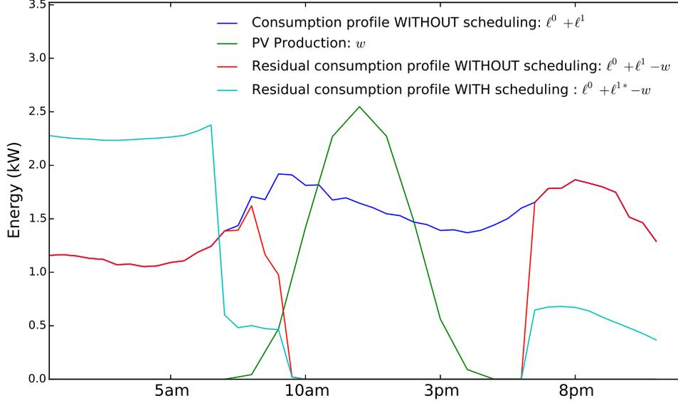
**Figure 13.** Daily energy consumption of flexible consumer with PV and storage. 8 PV panel are installed, the storage battery capacity is 7kWh.  $l^{1*}$  is the optimal scheduled flexible consumption profile. *Most of the energy need is removed to the late night.*
