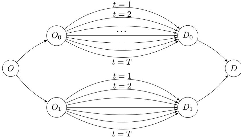
**Figure 2.** Network of the equivalent routing model. *The original arc  $O$  is the provider set, final arc  $D$  is the scheduled result for consumers, links from  $O$  to  $D$  are consumptions at each time slots  $t \in \mathcal{T}$ . Flows are atomic on the two first and last arcs and non-atomic on the two providers' sub-networks.*
