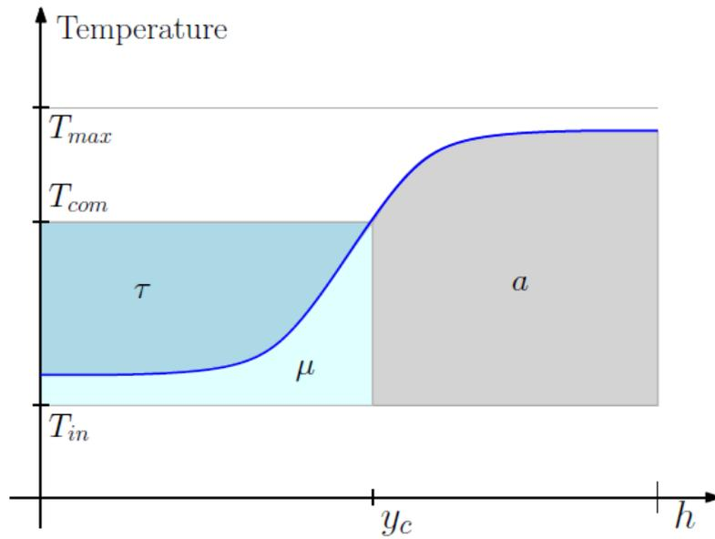
**Figure 3:** Temperature Profile, Available, Delay and Reserve Energy after a Drain
