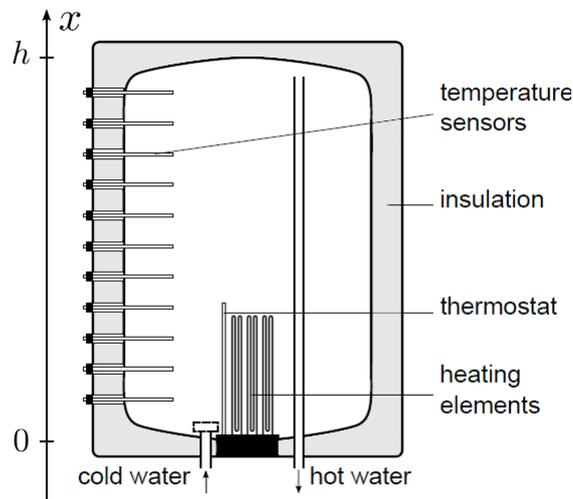
**Figure 2:** Schematic view of an electric hot water tank
