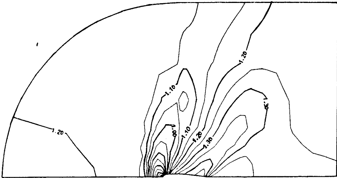
Figure 2.22 Courbes d'isomach, NACA 0012, M_\infty = 1.2 , \alpha = 0^\circ .
