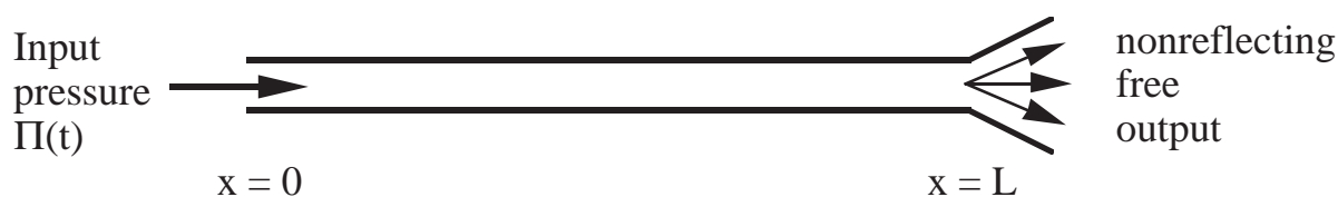
Figure 3.1. Long unidimensional pipe for the modelling of a trombone.
